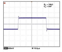
Figure 9. Output response of follower-connected OP1177 with capacitive load. Note high frequency ringing.
