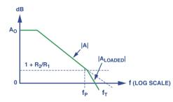
Figure 2. Bodé plot for the circuit of Figure 1.
