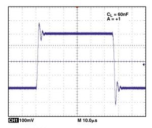
Figure 12. AD8698 output response without compensation.
