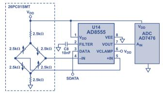
Figure 7. Pressure-sensing application example.
