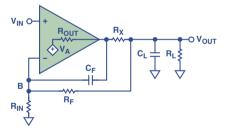
Figure 3. In-the-loop compensation circuit.
