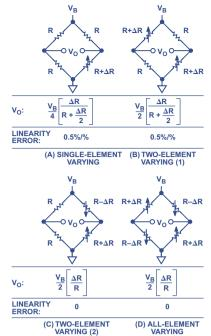
Figure 2. Bridge with four resistive elements.
