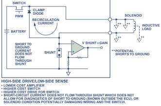
Figure 1. Electronic control unit with high-side switching and low-side sensing.
