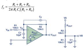
Figure 14. Capacitive loading at the input—inverting configuration.
