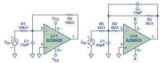
Figure 16. Input filter without (at left), and with (at right) compensation and lower impedance levels.
