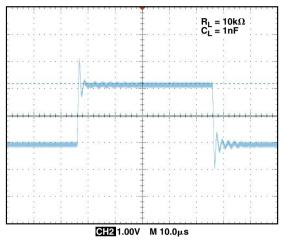
Figure 6. AD8510 output response without compensation.
