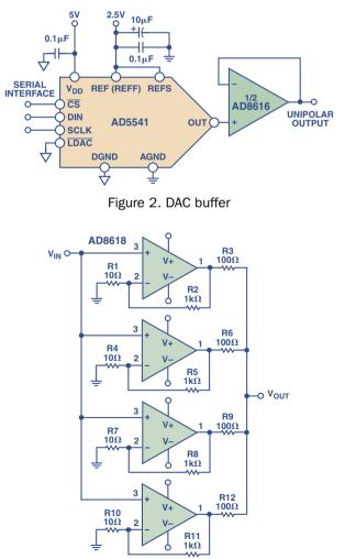
Figure 3. Noise reduction using multiple parallel paths
