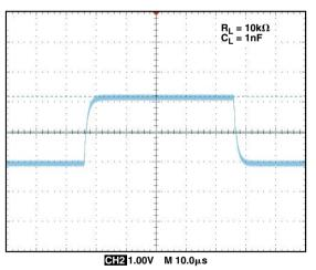
Figure 7. AD8510 output response with compensation.
